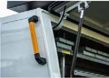
Grab Handle, Fitted To Body 200mm, black 300mm, safety yellow Safety grab handles provide additional point of contact to assist to step safety.
