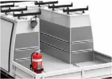
Chequer Plate Protection H600mm chequer plate. Protects external painted surfaces from tools of trade and equipment.
