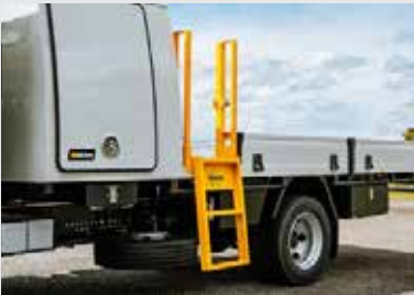
Folding Access Step W400 x H600mm W400 x H900mm W600 x H600mm Folding access step, in safety yellow, includes a 3 tier fold down step with anti slip finish on treads and LHS and RHS grab handle mullions to ensure 3 points of contact are maintained while accessing rear tray section.
