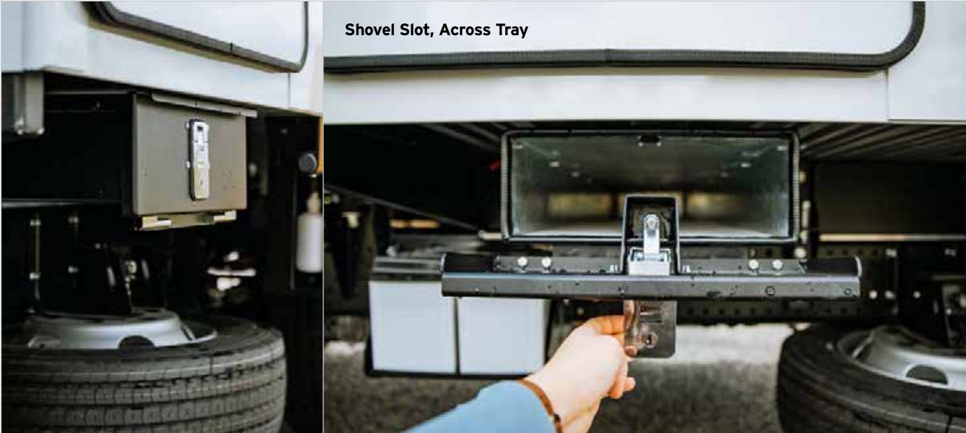
Underbody Box L450 x W300 x H450 mm L600 x W300 x H450mm L750 x W300 x H450mm L900 x W300 x H450 L1200 x W300 x H450 Truck underbody aluminum box, available in a range of sizes, are lockable and offer an additional secure storage space, making good use of under body space.
