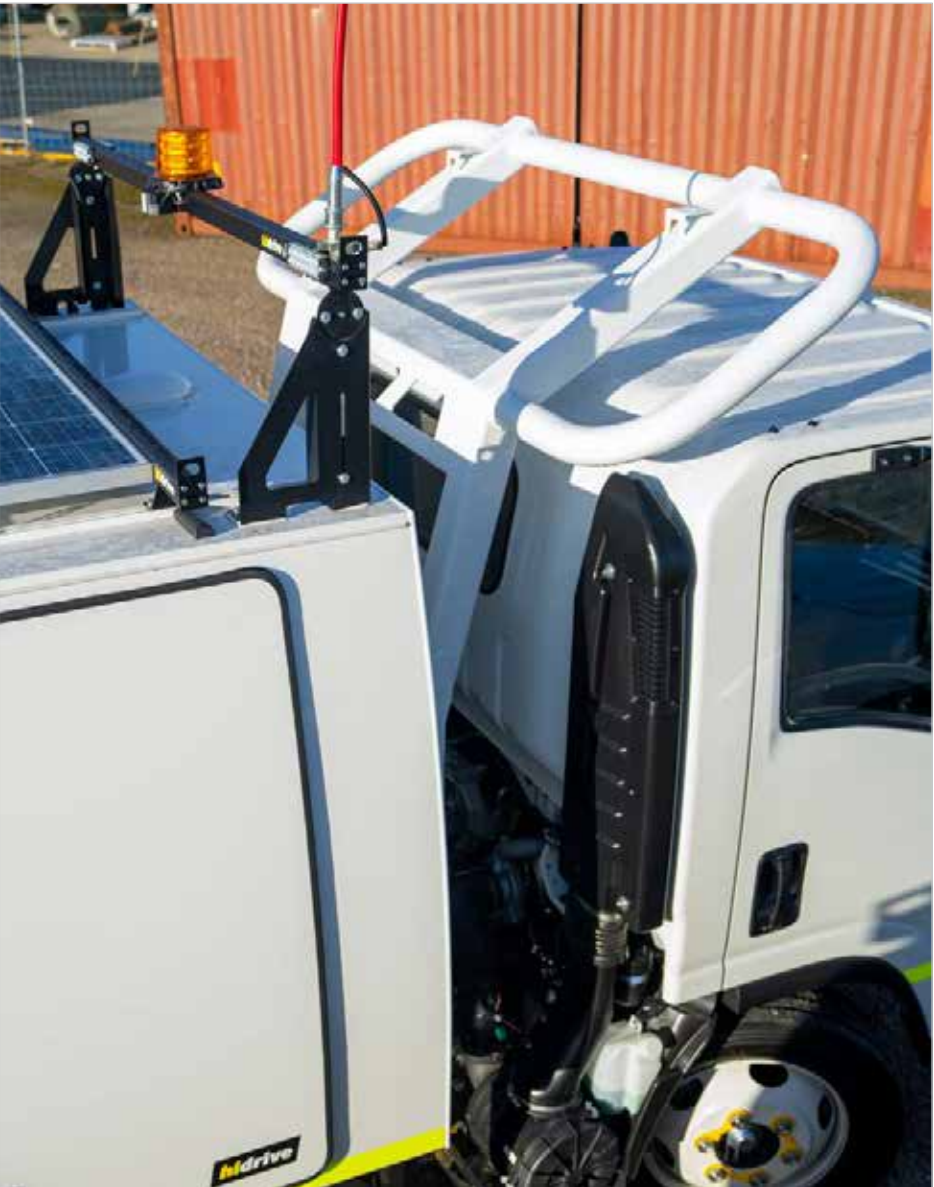
ROPS Cell, Vehicle Specific Roll over protection cell for safe compliant access to work sites. Only available on single cab truck variants.
