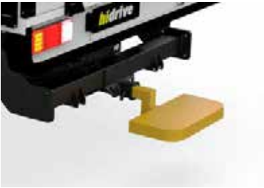
Rear Fixed Step, 500x25mm Hi-Vis safety colour. Fitted in place of towball. Assists safe access to rear tray area and rear roof accessories.
