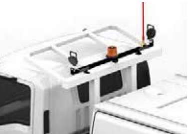
ROPS Cell, Vehicle Specific Roll over protection cell for safe compliant access to work sites. Only available on single cab truck variants.
