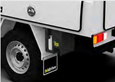
12L Water Tank, Underbody Box, Wheel Chocks & Bracket
