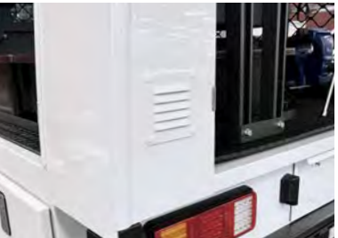
Louvre Vent Slim-lined, surface-mounted vent for side applications.
